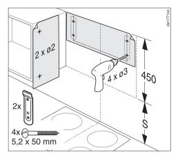
Cut the wall attachment drilling template and place it on the wall.
